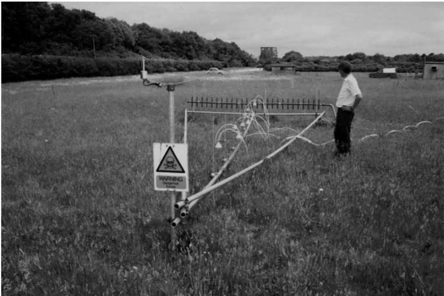
**Fig. 2.5** Andrew McLeod with an engineering prototype for release of  $O_3$  into FACE plots. Note the emitter jets facing outward toward vertical baffles. Photo by G. Hendrey
