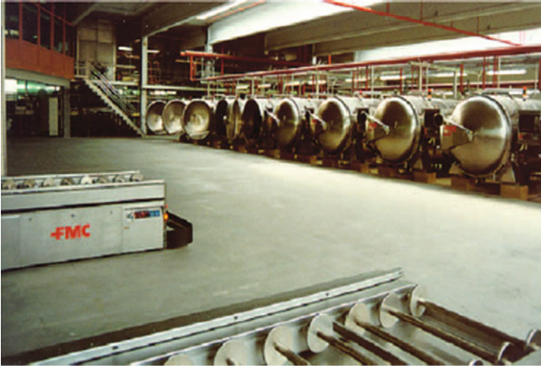
Fig. 21.4 Automated batch retort system with use of automated guided vehicles in large Cook room operation (Courtesy, FMC Food Tech., Madera, CA)
