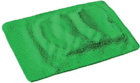
Fig. 6.9 Meshing of the 3D digitalized retort pouch
