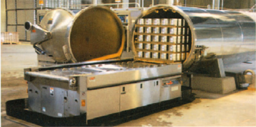
Fig. 21.5 Automated guided vehicle for batch retort loading/unloading (Courtesy, FMC Food Tech., Madera, CA)
