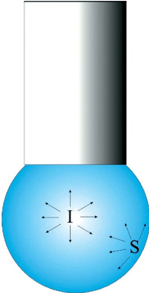
Fig. 4.1 Droplet of water at the end of a pipette. A molecule of water situated inside the droplet at “I” is attracted to its surrounding molecules by Van de Waal’s forces equally in all directions. A molecule on the surface at “S” would have more attractive forces inside rather than outside such that the resultant force is inwards. Surface tension therefore acts like a ‘tight skin’ trying to achieve the smallest surface area for a given volume
