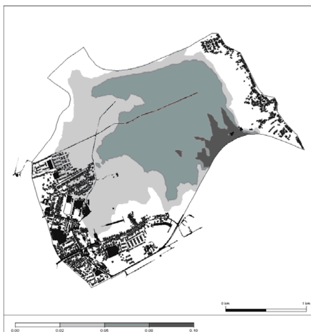
Fig. 4. Oil concentration [ \text{kg m}^{-2} ] in the simulation area at hydrodynamic steady state, 10 hours after start of flooding.
