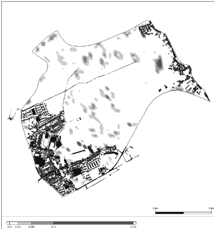
Fig. 3. Sediment accumulation [m] in the simulation area at hydrodynamic steady state, 10 hours after start of flooding.
