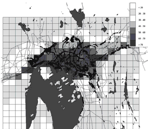
Fig. 4.2. The 8 th highest daily grid value of PM 10 ( \mu\text{g}/\text{m}^3 ) for Oslo in 2005. The black dots are illustrating the building points where the 8 th highest daily PM 10 value is above the national target of 50 \mu\text{g}/\text{m}^3 .
