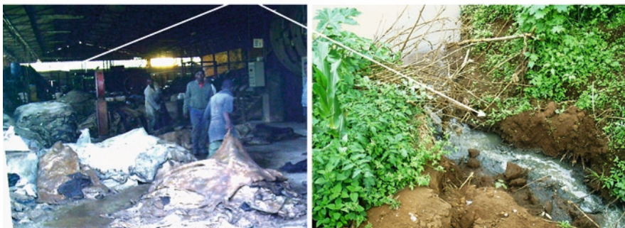
Fig. 2.1 Tannery operations with resultant chromium rich open disposal effluent systems
