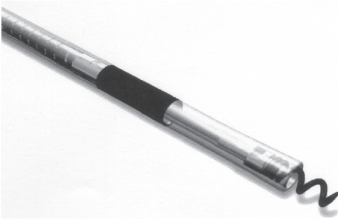
Fig. 1.19 Thin (4.1Fr) bipolar active-fixation lead with a fixed screw and no lumen for a stylet. (Medtronic 3830 SelectSecure™). The screw is coated with beclomethasone. The lead is delivered by a steerable catheter. (Permission for use: Medtronic.)
