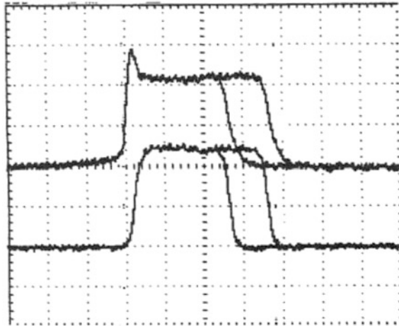
Fig. 29.2 Typical oscillograms of voltage (upper trace) and current (bottom trace) for two different voltage pulse durations (see Fig. 29.1). The time scale is 100 ns/div
