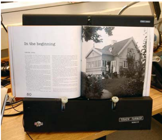
Fig. 12.6. Electric-powered page turner
