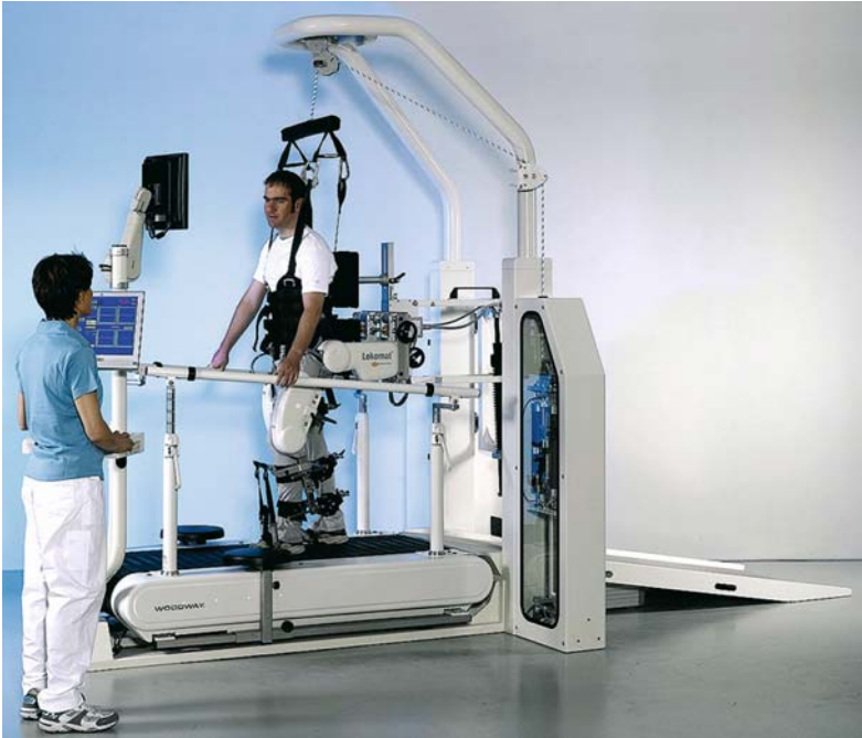
Fig. 12.2. Similar parachute-like harness together with adjunctive robotics (the Lokomat system) was developed by Swiss company, Hocoma
