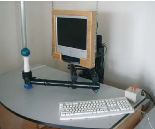
Fig. 6.13. Robotic arm developed at MIT in Boston, can potentially aid in the rehabilitation of patients with upper extremity disability
