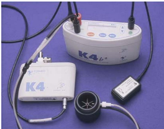
Fig. 8.15. Instrumentation for assessing oxygen consumption
