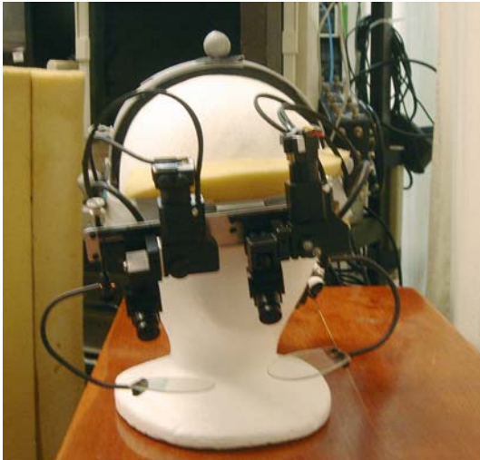
Fig. 19.7. Optical tracking device used in some research laboratories for investigation of falls
