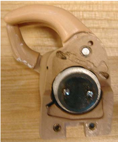
Fig. 10.15. Myoelectric wrist unit for the child amputee
