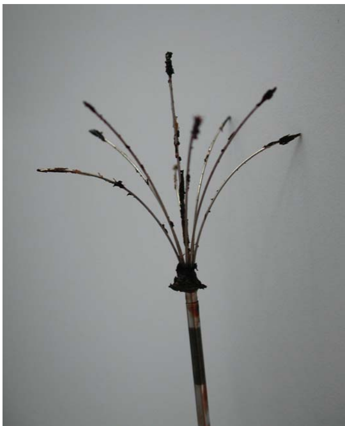
Fig. 8.7 Charred lung tissue sticking to the electrodes
