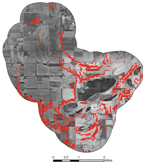
Fig. 7.2 The Revised Universal Soil Loss Equation (RUSLE) was used to estimate soil erosion in the Rainwater Basin. Red areas are those with predicted soil loss greater than 5 tons/acre/year
