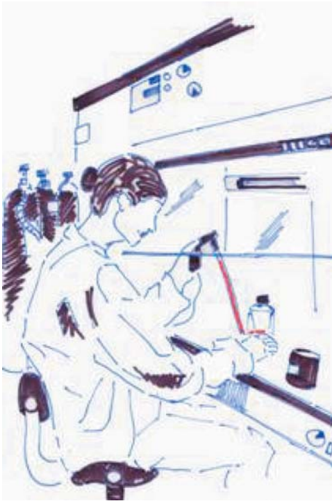
FIGURE 4.1. Cell culturing in a laminar flow cabinet. Note the scientist is using a battery-operated “pipette boy” to draw the media up into the pipette. (Courtesy of P.N. Vaiude, Honorary Clinical Fellow, Barts and the London NHS Trust.)
