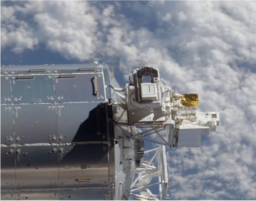
**Fig. 2.7** SOLAR, an ESA observatory on the Columbus laboratory which forms part of the International Space Station. It carries three complementary instruments which make measurements of the Sun’s spectral irradiance from 17 to 100 nm, within which 99% of the solar energy is thought to be emitted
