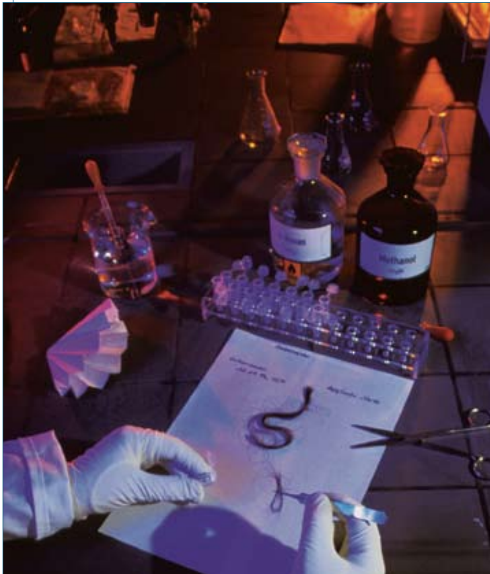
FIGURE 3.1 A hair sample from a suspected drug user is prepared for forensic analysis. As hair grows, it incorporates small amounts of chemicals that are produced when drugs are broken down in the body. To identify these drugs, the hair is first cut into pieces and soaked in a liquid solvent. The solvent removes the traces of drug metabolites from the hair so that they can be identified by chromatography and mass spectrometry.
