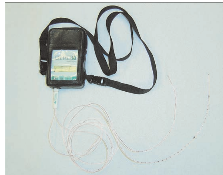
2.31 A triple pH probe with portable data logger. The data loggers use sampling rate of eight per minute with 0.1 pH unit resolution. There are input buttons on the data logger to indicate events such as heart burn, meal time, supine position, and so on.
