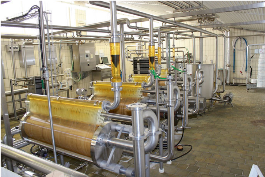
Fig. 5.4 Ultrafiltration of modern skyr (©MS Selfoss, Iceland)
