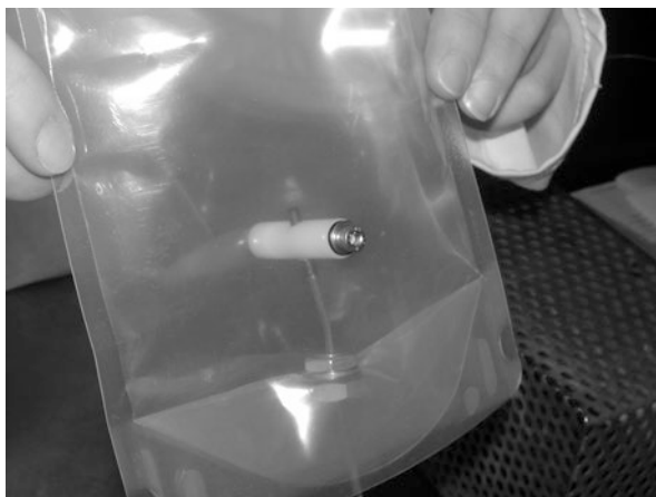
Fig. 10.3 Thermocouple held in place in retortable pouch
