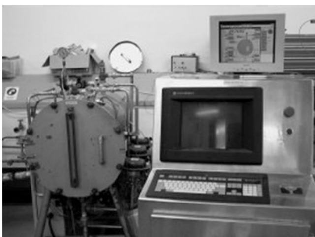
Fig. 10.5 Automatically controlled and monitored retort (steam pressure vessel)
