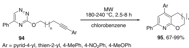
Scheme 2.67 Intramolecular inverse electron demand Diels–Alder reactions under MW irradiation
