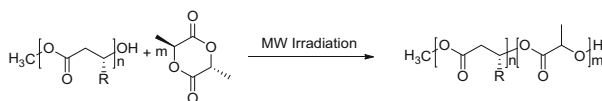
Scheme 3 Synthesis of PHA- block -(PDLA- stat -PLLA) diblock copolymers after initiation of the R,S -lactide polymerization by a poly(hydroxy alkanate) macroinitiator
