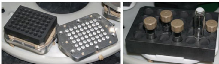
Fig. 6 A 48-position ( left ) and a 24-position ( right ) silicon carbide plate capable of holding standard glass vials
