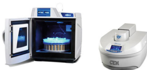
Fig. 3 A (larger) multimode ( left ) and a (smaller) monomode ( right ) scientific microwave unit (Reproduced with permission from CEM Corporation)
