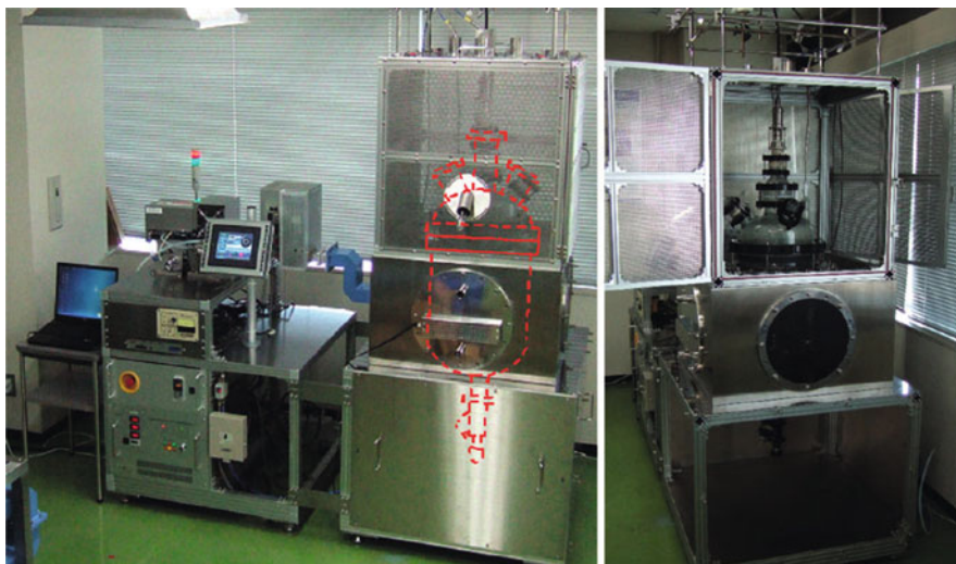
Fig. 4 Pictures of the SMW-114 MW reactor showing the entire instrument ( left ) and the reaction cavity ( right ). Reprinted with permission from [42]
