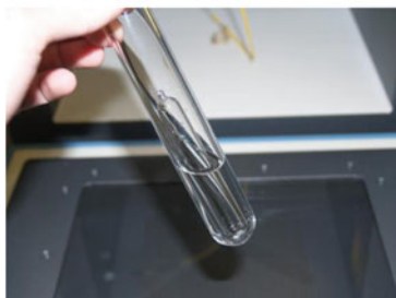
Fig. 5 Electrodeless discharge lamp inside the reaction vessel used for performing microwave irradiation in conjunction with UV irradiation ( left ) and the vessel assembly in use ( right )
