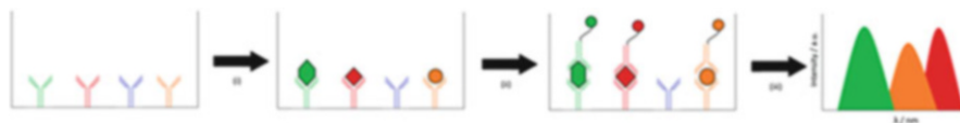
Fig. 4 Schematic illustration of a multiplexing fluorescence immunoassay using QDs with three distinct emission colours. Capture antibodies are fixed to the bottom of a well and (i) antigen mixture added followed with a wash step (ii) reporter antibody-QD conjugates added followed by wash step (iii) fluorescence intensities analysed of each specific QD
