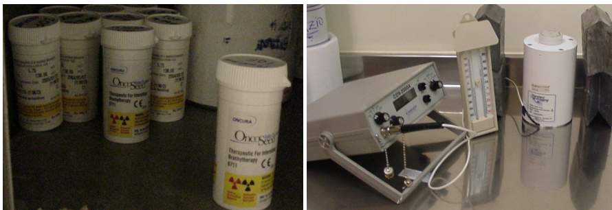
Fig. 6. Dosimetric verification of seeds for implant. Seed container (left). Measurement of each seeds using a well chamber (right).
