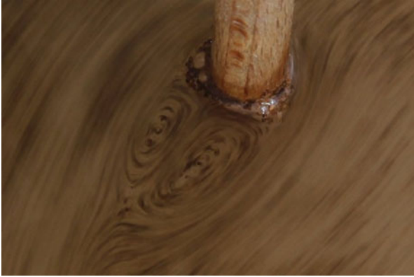
Fig. 4.7 A glimpse at unsteady recirculating vortices behind a cylinder at Re \sim 330 (photo of the author)
