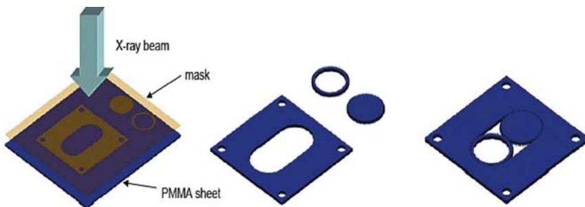
FIGURE 4.5. Standard DXRL fabrication process of the micro gearpump on a self-standing PMMA foil.
