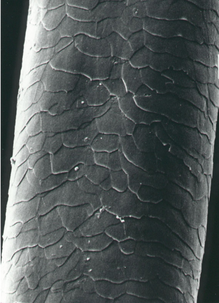
Fig. 8.2 Scanning electron microscope (SEM) micrograph of a human hair fiber
