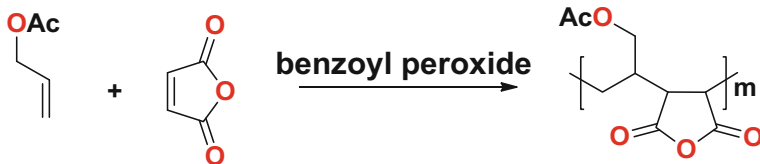
Scheme 4.3 Equimolar copolymerization of maleic anhydride and allyl acetate (adapted from [40])
