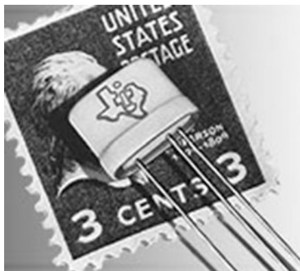
Fig. 9.27 1954 Texas Instruments' advertisement for the silicon transistor [62], used with permission from Texas Instruments Incorporated
