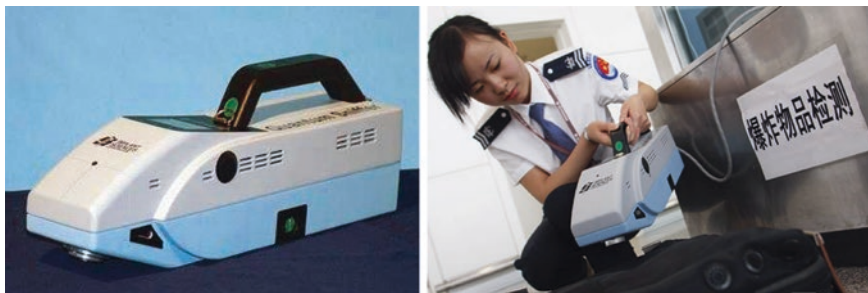
Fig. 2.9 An example of a suitable effluence detection device—the Quantum Sniffer QS-H150 Portable Hand-held Explosives Trace Detector ( anjian110.com )
