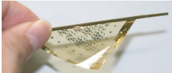
Fig. 15.2 Flexible circuit [5] (Reproduced with permission from Ref. [7]. Copyright 2010 Nature Publishing Group)
