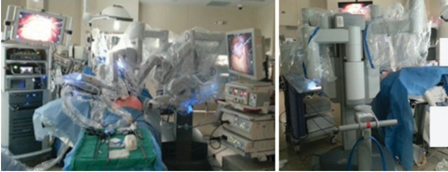
Fig. 18.3 Robotic patient side cart. Demonstrated is an intra operative photograph demonstrating the da Vinci SI system. Note the parallel side dock technique which allows for easy access to the head of the patient for anesthesia as well as for intra operative endoscopy. Figure reproduced from: Shah SK , Walker PA, Snyder BE, Wilson EB. Chapter 6: Essentials and future directions of bariatric surgery. In: Kroh M, Chalikhonda S (eds) Essentials of Robotic Surgery, Springer Science + Business Media, New York. 2015
