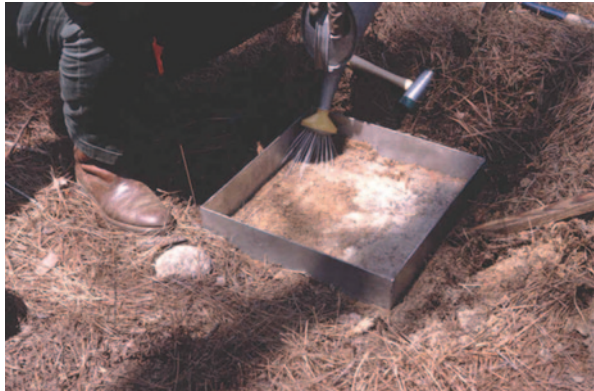
Fig. 12.4 Termiticide application to a ground board plot
