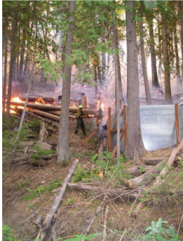
Fig. 21.17 Sediment catchments were established at the mouths of eight small watersheds at the Priest River Experimental Forest to test the effects of prescribed wildfire (shown) and wildfire followed by logging on soil, vegetation, and water properties
