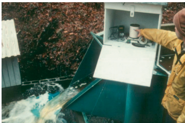
Fig. 15.8 Monitoring installation used to measure streamflow amount and collect water samples on Watershed 11 in the Alum Creek Experimental Forest. Device being pointed to records the water depth on a paper chart while the device immediately to the left records the same data in a digital file
