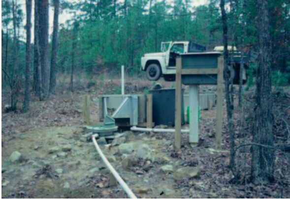
Fig. 15.9 Installation for measuring sediment production from a forest road. Equipment is the same as that shown in Fig. 15.5 and 15.8, but has an extended approach section between the flume and the road which collected the bed load sediment eroded from the road. Total sediment was the combined amount deposited in the approach section and the suspended portion that flowed over the flume and was measured using the Coshocton wheel samples
