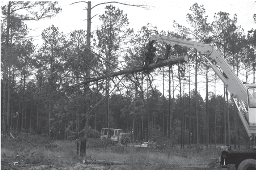
Fig. 23.4 Full-tree suspension of trees by a loader to avoid machine traffic and possible soil compaction at the Palustris Experimental Forest installation
