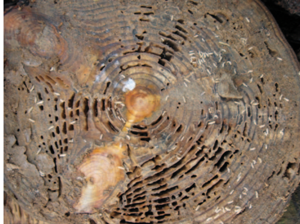
Fig. 12.1 Subterranean termites and their damage to a pine bolt
