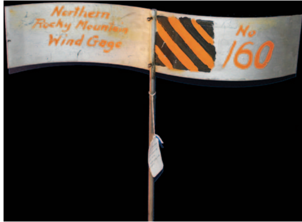
Fig. 21.6 An anemometer that George Jemison calibrated while riding on a hood of a car as his wife drove. Note each gage was numbered
