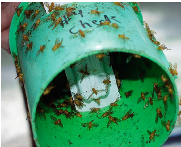
Fig. 13.13 Cylindrical bait station made of a polyvinyl chloride (PVC) pipe (10.1 cm internal diameter and 10 cm in length) with a conical top and supported bait tray inserts that can be filled with protein-based bait for efficient storage and transport (Mangan and Moreno 2007) (Photo: R. Mangan)
