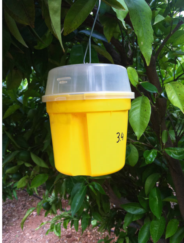
Picture 15.9 Moskisan with lateral chimneys and invaginated hole in the bottom of the trap
