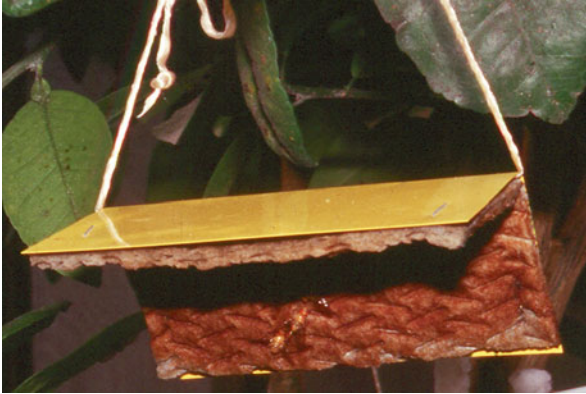
Fig. 13.12 Tent-shaped bait station consisting of a sheet of sponge attached under a folded sheet of plastic (21.5 by 24.0 cm) folded in half to make 90° angle. The sheet of sponge material (19 by 20 cm and 8 mm in thickness when baited with a protein-based attractant) was stapled to the underside of the tent to line the under surface leaving a 2.0-cm overhang of the plastic on all sides. Developed by Mangan and Moreno (Mangan and Moreno 2007) and tested against Anastrepha ludens (Photo: R. Mangan)
