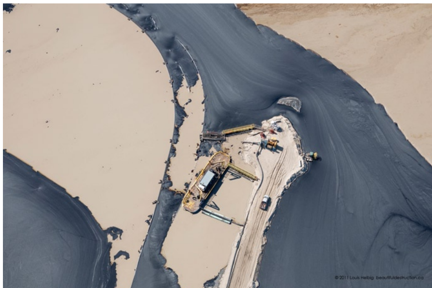
Fig. 5.6 Sound Cannon N 56.54.51 W 111.23.04, Suncor Millennium Mine, Alberta, Canada. With permission. Layers of thick Bitumen surround a sound cannon and other equipment at the edge of a tar pond. The sound cannons are designed to deter birds from landing in this toxic water. www.louishelbig.com/
