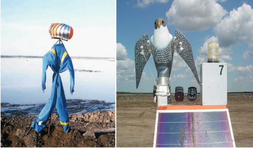
Fig. 5.5 Bird deterrent technology in use on tar sands tailings ponds ranges from glorified scarecrows to robo-hawks equipped with radar detection. Photos courtesy of Colleen Cassidy St. Clair
