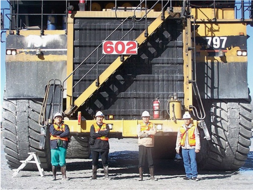
Fig. 3.27 September 2005 , 08:20. Caterpillar 797 truck empty weight: 557,820 kg (1,230,000 lb). Drive: 3524B EU1 twin turbocharged and after cooled diesel engine. Max speed: 64 km/h or 40 mph. Horse power: 3,500. Suspension: self-contained oil pneumatic suspension cylinder on each wheel. Height empty: 7.1 m (23 ft 8 in.), length: 14.3 m (47 ft 7 in.), body width: 9.0 m (30 ft). Dumping height: 14.8 m (49 ft 3 in.). Tire size: 3.8 m (12.9 ft) in diameter. Cost: $5–6 million Creative Commons. See also Peter Essick, http://s.ngm.com/2009/03/canadian-oil-sands/img/candian-oil-sands-truck-160.jpg
