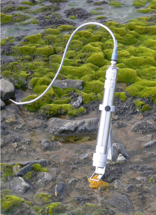
Fig. 20.11. Field installation of a fluorometer for long-term measurements of effective quantum yield of photosynthetic processes in Xanthoria elegans (James Ross Island, Antarctica) (Photo M. Barták).
