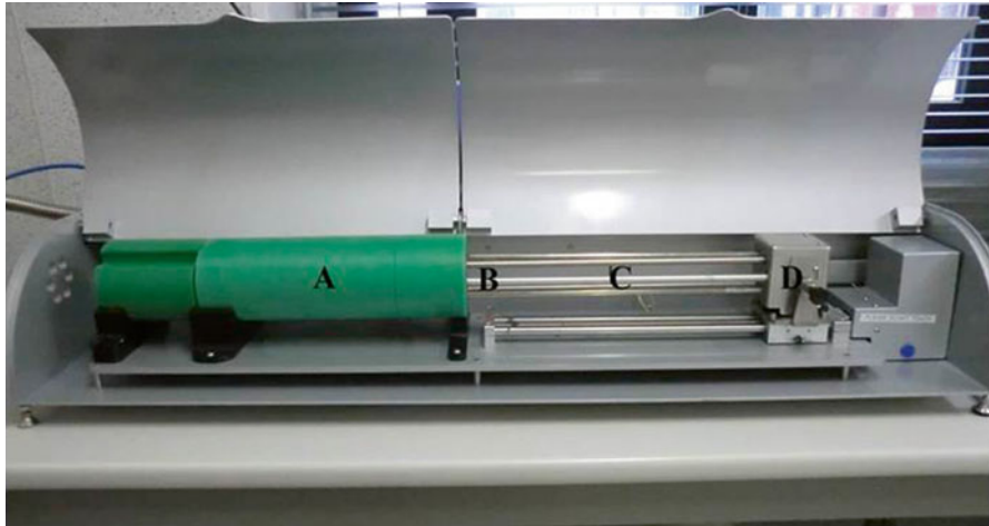
Fig. 9.2 The Multi-Thermal-Gradient (MTG) freezing device. (A) cooling block; (B) entrance of the sample's glass tube; (C) metal rod, which advances the sample's glass tube forward into the cooling channel in the cooling block; and (D) electric motor
