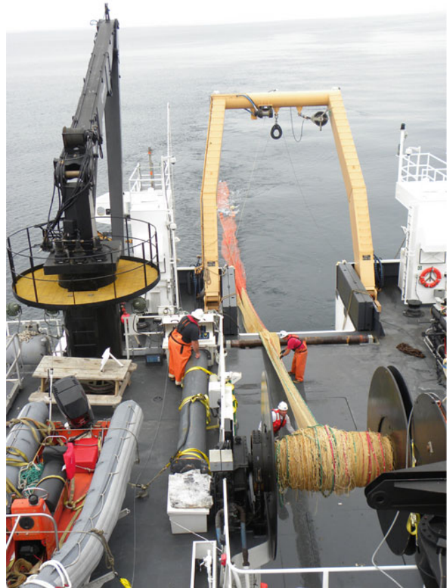
Fig. 3.3 Nordic 264 rope trawl being deployed from Bell M. Shimada, October 2010. Normally this trawl is fished near the surface at night to obtain dispersed small pelagic fishes (Photo: S. McClatchie)
