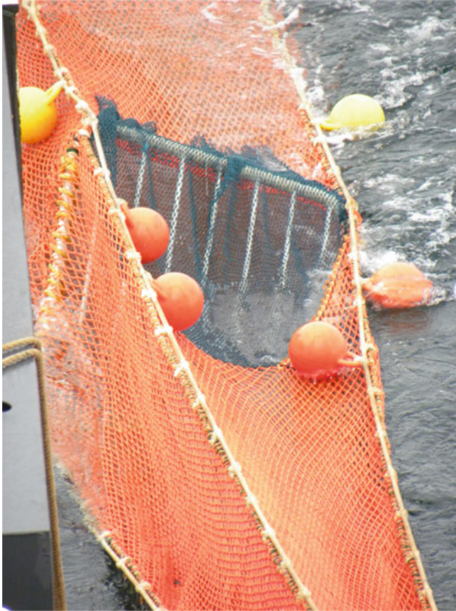
Fig. 3.4 Marine Mammal Excluder Device (MMEL) sewn into the Nordic 264 rope trawl to permit escape of inadvertently entrained bycatch such as seals, sea lions and dolphins (Photo: D. Griffith)
