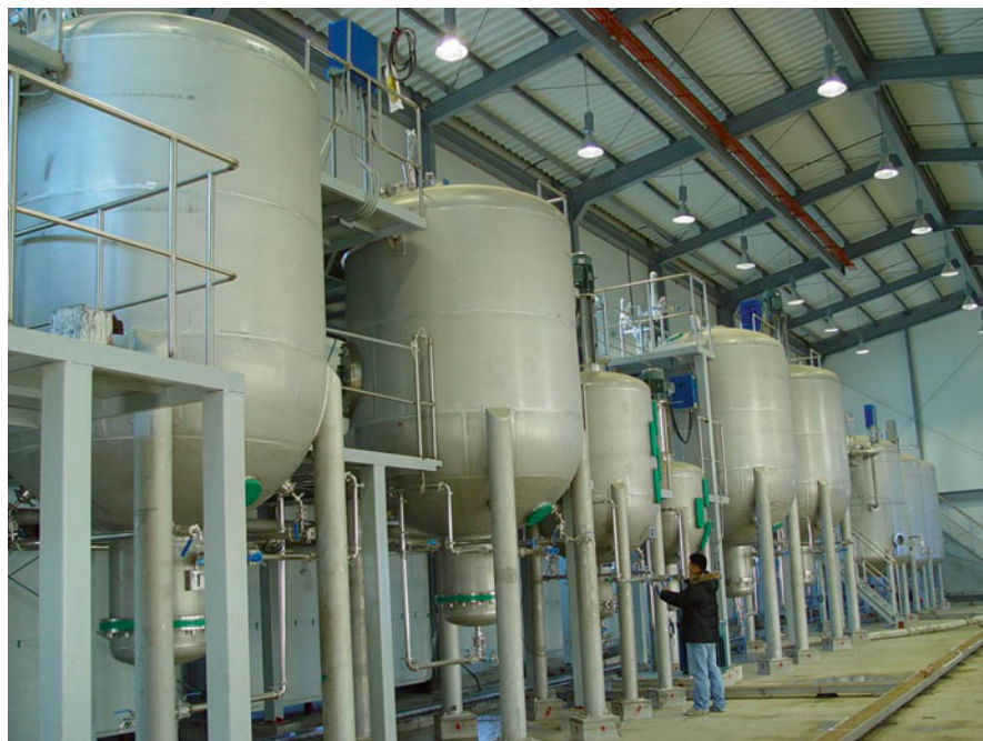
Fig. 20.12 Large-scale (10,000 L) bioreactors developed for cultivating adventitious roots of ginseng
