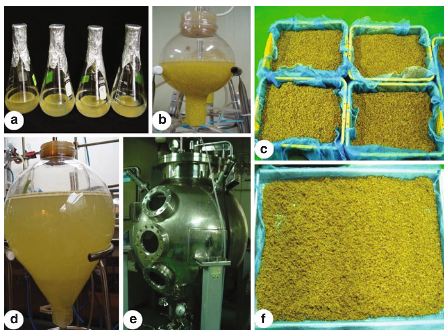
Fig. 13.3 Suspension cultures of somatic embryos of Eleutherococcus senticosus : (a) Embryogenic cells in MS liquid medium supplemented with 30 g sucrose L -1 and 1.0 mg 2,4-dichlorophenoxy acetic acid L -1 . (b) Embryogenic suspension in 3 L capacity balloon-type airlift bioreactor containing 2 L MS medium with 30 g sucrose L -1 . (c) Biomass harvested from 500 L balloon bioreactor after 30 days of culture. (d) Embryogenic suspension in 20 L balloon type airlift bioreactor. (e) Embryogenic suspension in 500 L balloon-type airlift bioreactor. (f) Biomass harvested from 20 L balloon bioreactor after 30 days of culture
