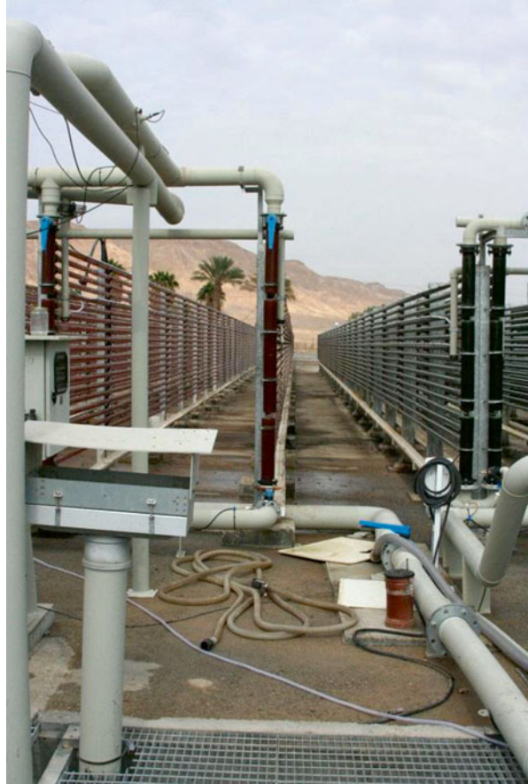
Fig. 4.5 Cultivation of H. pluvialis in tubular photobioreactor (Algatech, Israel). Note the tubular fences with green vegetative cell suspension ( right ) and those with red astaxanthin-rich cysts ready for harvest ( right ) (Photo: A. Solovchenko)
