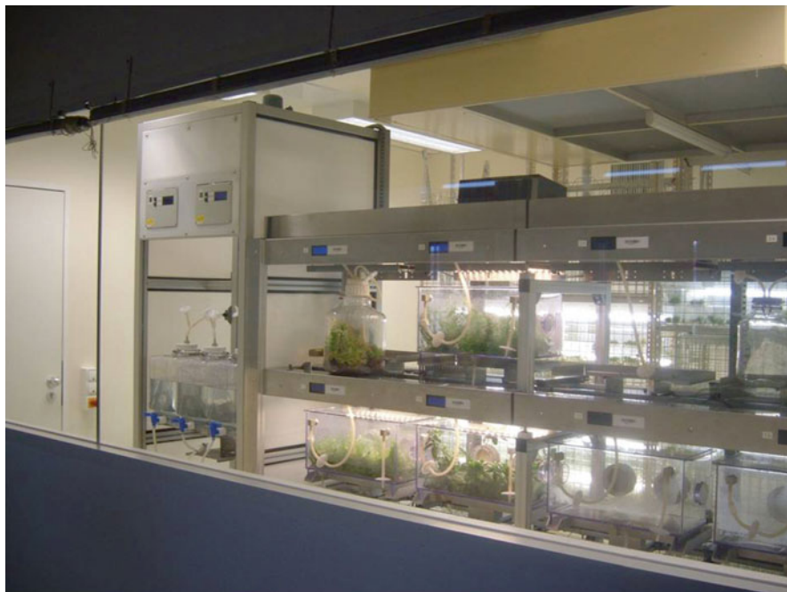
Fig. 17.4 Automation of an industrial applicable culture system for bioreactors
