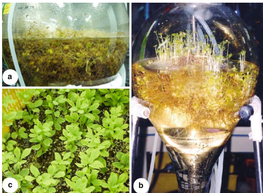
Fig. 14.7 Plantlets production via somatic embryogenesis in a 20 L air lift bioreactor, (a) Embryo formation after 4 weeks of culture in one third MS medium containing 60 g L -1 sucrose, (b) Plantlets in bioreactor after 12 weeks of culture, (c) Plantlets grown on the peat moss and perlite mixture after 8 weeks of acclimatization (Adapted from Park et al. [10])
