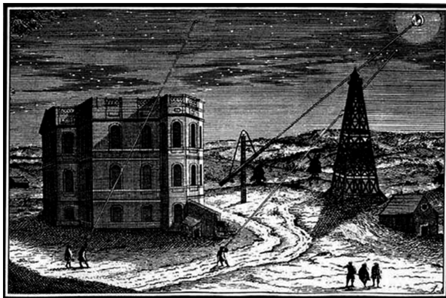
Fig. 3 A woodcut showing observers in the foreground, in front of the Paris Observatory, using two of the very long focal length refractors. Their objectives were attached to the Observatory building itself (in the case of the left-hand pair of observers) and to the Marly Tower (in the case of the right-hand observer). The lines apparently joining the objectives and the eyepieces in this woodcut are there to indicate the incoming light rays, not tubes, as these telescopes lacked tubes (indeed these were referred to as ‘telescopes without tubes’ by Cassini). Meanwhile, the much shorter focal length telescope in the background, on the terrace and attached to the mast, does have a tube (After Wolf 1902)
