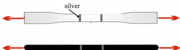
Fig. 4.8 Two different possible shapes for a composite specimen for tension and compression tests
