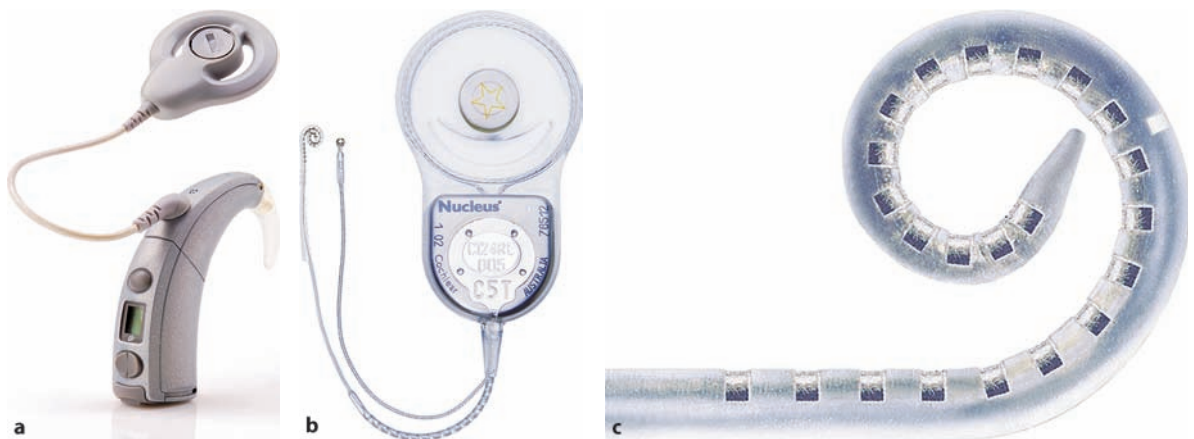
Fig. 45.1a–c Example of a cochlear implant. a External parts: speech processor, which contains the microphone, battery, and electronics to receive the electrical signal from the microphone, manipulate it, and change to a radio signal, for transmission across the scalp. The cable leads to the transmitting aerial, with a central magnet to couple with the implanted magnet and hold the aerial in place on the scalp. b The implanted part of a typical cochlear implant. The receiving aerial, with a central magnet (to couple with the external magnet shown in a ). This leads the signal into the main implant package, which decodes the radio signal, converts it back into an electrical signal and sends it down the main cable, terminating in 22 active electrodes. There is also a single, ball-shaped, indifferent electrode, which is placed deep to the temporalis muscle. c An enlarged view of an intracochlear electrode array. There are 22 active electrodes, which lie in the scala tympani and the shape of the array holds it coiled close to the modiolus
