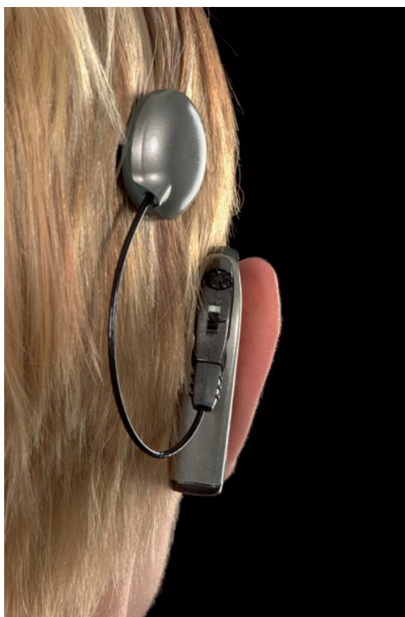
Fig. 45.2 Photograph of a typical multichannel cochlear implant in place. The speech processor is hooked behind the pinna. The external transmitting aerial is held magnetically against the scalp and exactly over the internal receiving aerial
