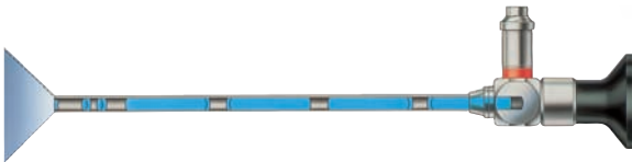
Fig. 20.4 A Storz rigid telescope, using the Hopkins rod system
