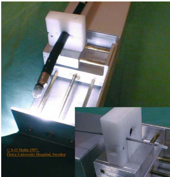
Fig. 23.10. A prototype acquisition unit for 3D EUS imaging that can be used both for echoendoscopes and miniprbes. The pullback system allows for a constant speed of transducer movement
