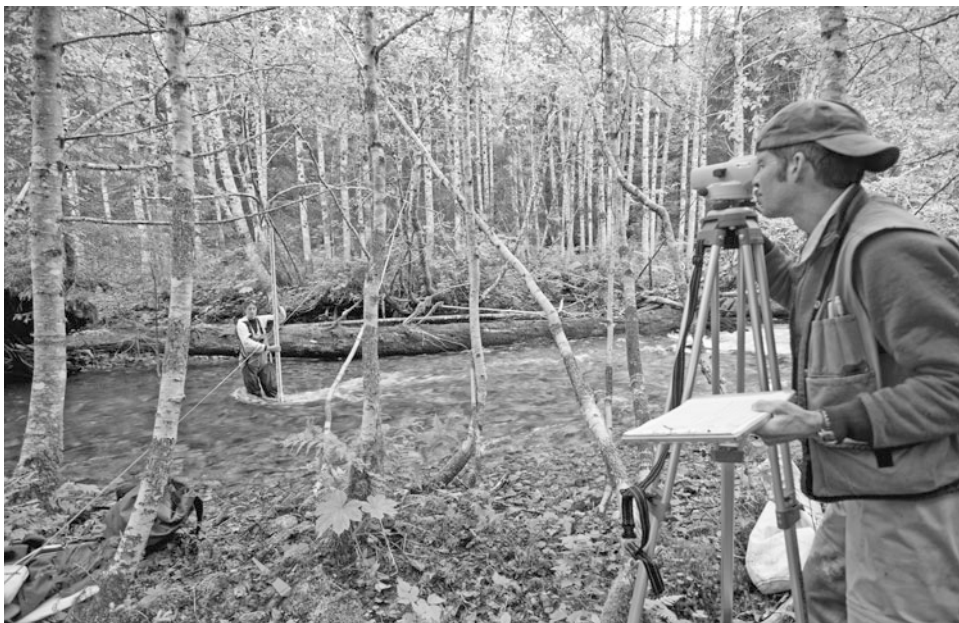
FIGURE 9.3. U.S. Forest Service hydrologists monitoring water depth at Kennel Creek, Tongass National Forest. (Photo courtesy of Bob Christensen)
