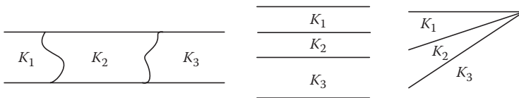
FIGURE 7.8 Hydraulic conductivity formations in three types of heterogeneous systems.
