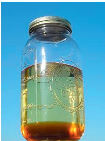
**Figure 1.9** A batch of home-made canola oil biodiesel sitting on top of its glycerol layer (photo courtesy of Biodieselcommunity.org).
