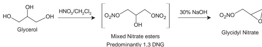
**Figure 7.9** The continuous process for the production of glycidyl nitrate, and thus PGN, from glycerol involves consecutive nitration and caustication.
