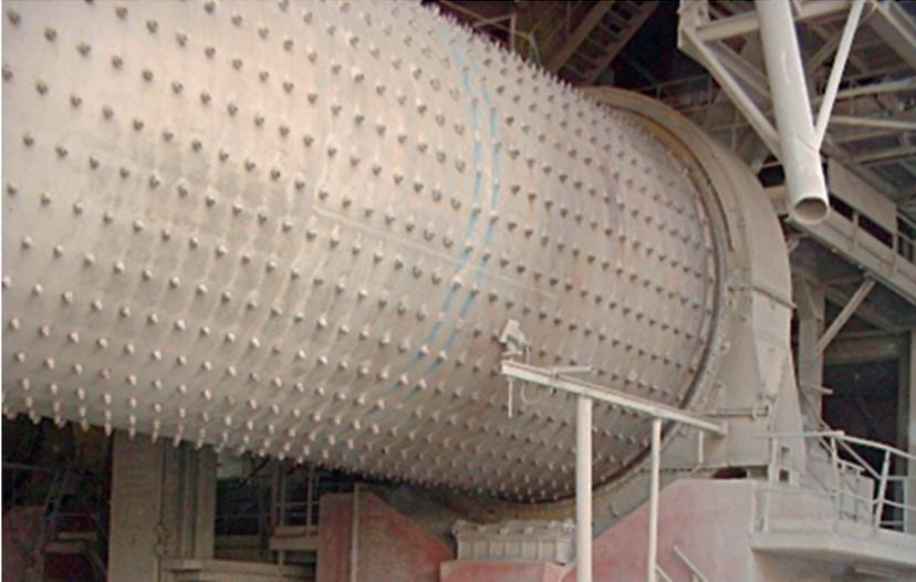
**Figure 9.4** A ball mill used to grind clinker and produce cement (photo courtesy of Grace Construction Products).
