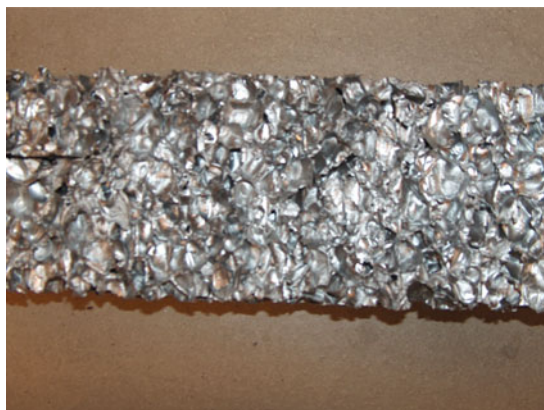
Fig. 14.29 Aluminum foam core
