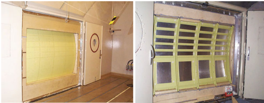
Fig. 14.53 Mounting of Panel F. Left picture as seen from the reverberation room, right picture from the anechoic room
