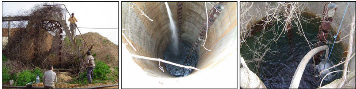
Fig. 11 Injection test developed in the “nora”: water levels at the beginning and at the end of the test
