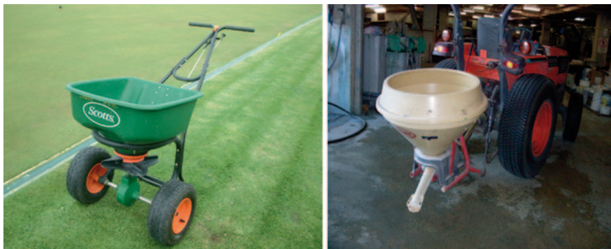
Fig. 22.2 Granular fertilizer application can be carried out by drop-type (gravity) spreaders or rotary-type (centrifugal) spreaders
