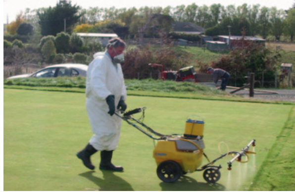
Fig. 22.9 Wear protective clothing and equipment mentioned on the label. Read the label in regard to health and safety concerns in spray application
