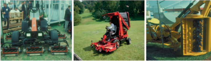
Fig. 22.1 The main mechanised mower types include the cylinder or reel ( left ), rotary ( middle ), mulch and flail mowers ( right ). Rotary mowers use a rotating blade or blades to cut vegetation with mulching technology introduced for use with rotary mowers
