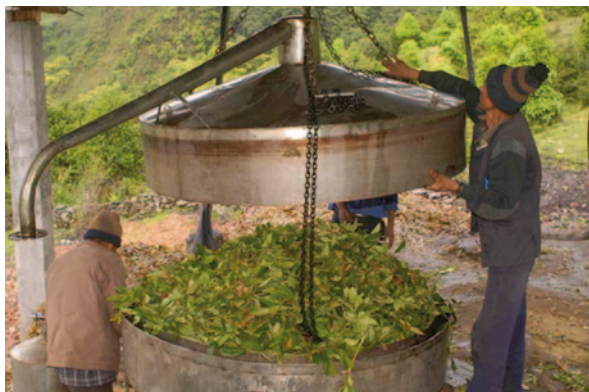
Fig. 18.2 Preparing for distillation of essential oil in Nepal. (Source: Photo courtesy of Han Saran Karki)
