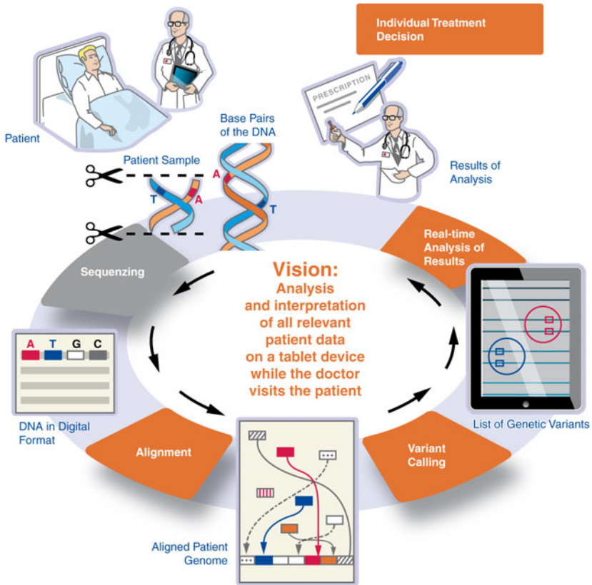
Fig. 1.1: Data processing steps involved in the analysis of genome data. Sequencing the samples results in chunks of DNA are available in digital form. During alignment their position within the whole genome is mapped. Variant calling results in a list of differences of a fixed reference. The analysis obtains new insights based on the list of detected variants.
