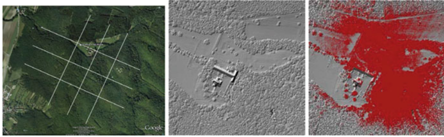
Fig. 2.11 Orthophoto of the study site “St. Anna in der Wüste” (left) with hillshade of the area around the former monastery, derived from FWF ALS data (centre) and overlaid TLS coverage in red (right) (From Doneus et al. (2010))
