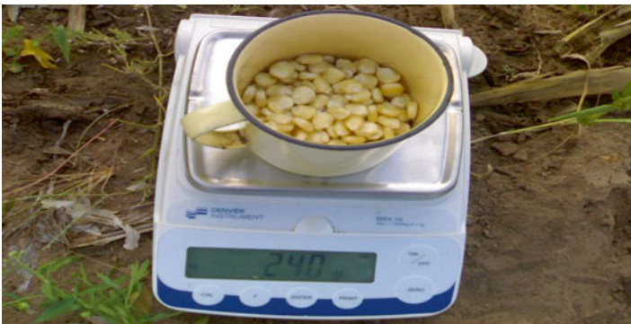
Fig. 7.7 Measuring grain moisture content
