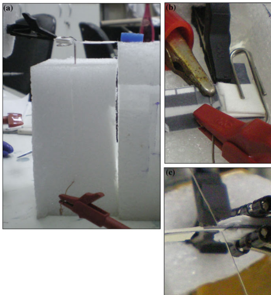
Fig. 2.12 Some of the approaches used for electrode positioning. a with a sponge support, b with a Pt wire stacked across the width of the channel, c with a Pt wire passing through paper
