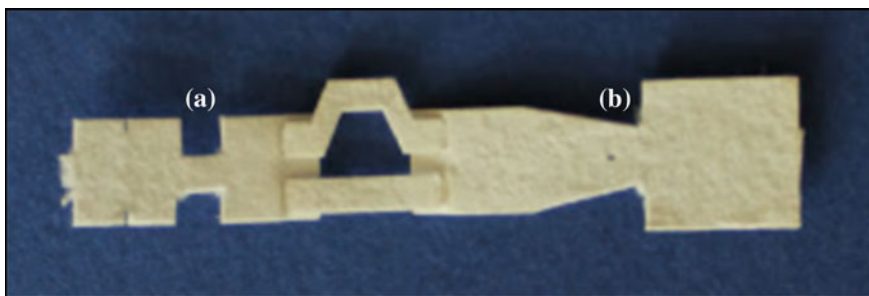
Fig. 2.16 Device with partially constricted channels. a sampling constriction, b electrode constriction
