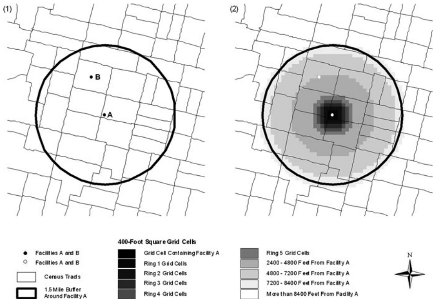
Fig. 19.1 Illustration of the distance decay method
