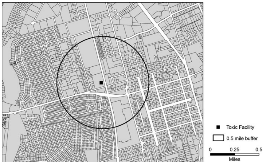
Fig. 5.6 Cadastral dasymetric mapping: using land parcels to estimate households within a buffer
