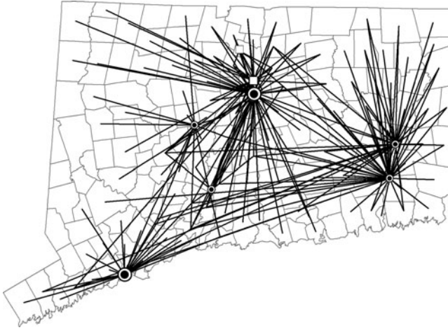
Fig. 12.6 Direct flows of municipal solid waste to trash-to-energy plants and landfills from town centroids
