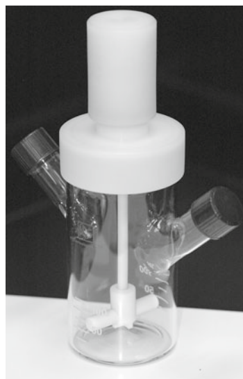
Fig. 1 Stirred suspension bioreactor [SSB] (125 mL)
