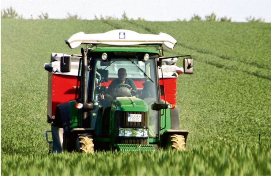
Fig. 9.25 Control of nitrogen spreading via reflectance sensing based on artificial light with oblique viewing of the canopy from the roof of the tractor (From Agri Con GmbH, Jahna, Germany)
