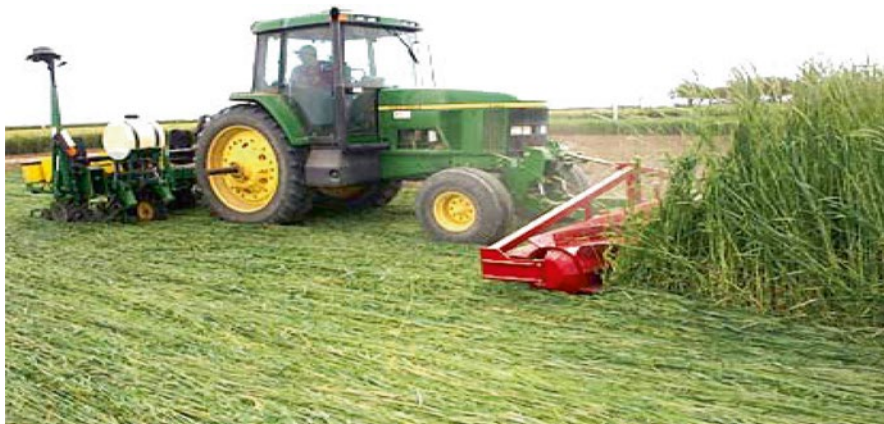
Fig. 8.13 Roller-crimper in front of a tractor for no-till seeding into a cover crop. The metal strips on the roller drum crimp the stems. They should not cut or chop the stems (Courtesy of I & J Manufacturing, Gap, Pennsylvania)
