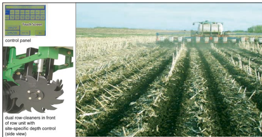
Fig. 8.11 Field sown with maize after maize without any previous cultivation by using row cleaners in front of the seeding units ( right ). The insert ( left ) shows a row cleaner for site-specific depth control in front of a seeding unit (Courtesy of Yetter Mfg. Co. Inc., rearranged and altered)
