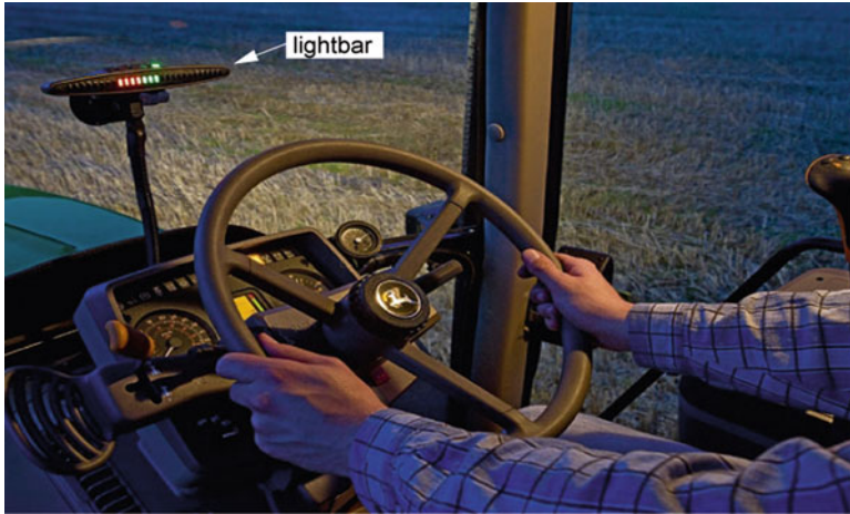
Fig. 4.4 Manual guiding assisted by lightbar indications (From John Deere & Co., altered)
