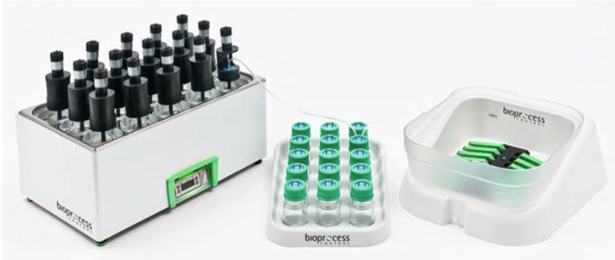
**Fig. 8** Automatic methane potential test system (AMPTS) for monitoring BMP of up to 15 samples simultaneously. Material to be evaluated is mixed with an inoculum, and the gas formed is passed via a scrubber where  $\text{CO}_2$  and  $\text{H}_2\text{S}$  are removed. The remaining gas is fed to gas flow meters. Courtesy: Bioprocess Control AB, Lund, Sweden
