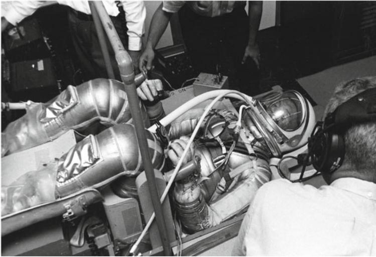
Joe Schmitt conducts a suit pressurization test. (Photos: NASA)
