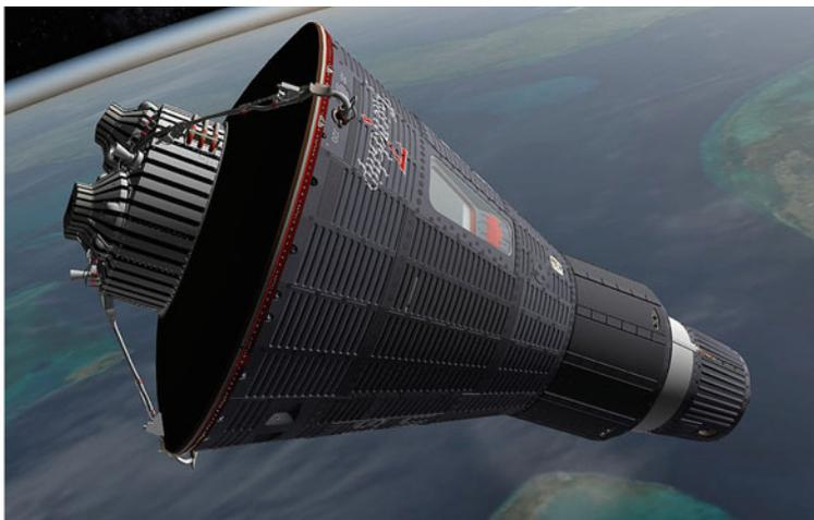
A reproduction of *Friendship 7* in orbit, showing the blunt-end heat shield and the retro-package attached to the rear of the spacecraft. (Image generated with Celestia; 3D model created by James R. Bassett)
