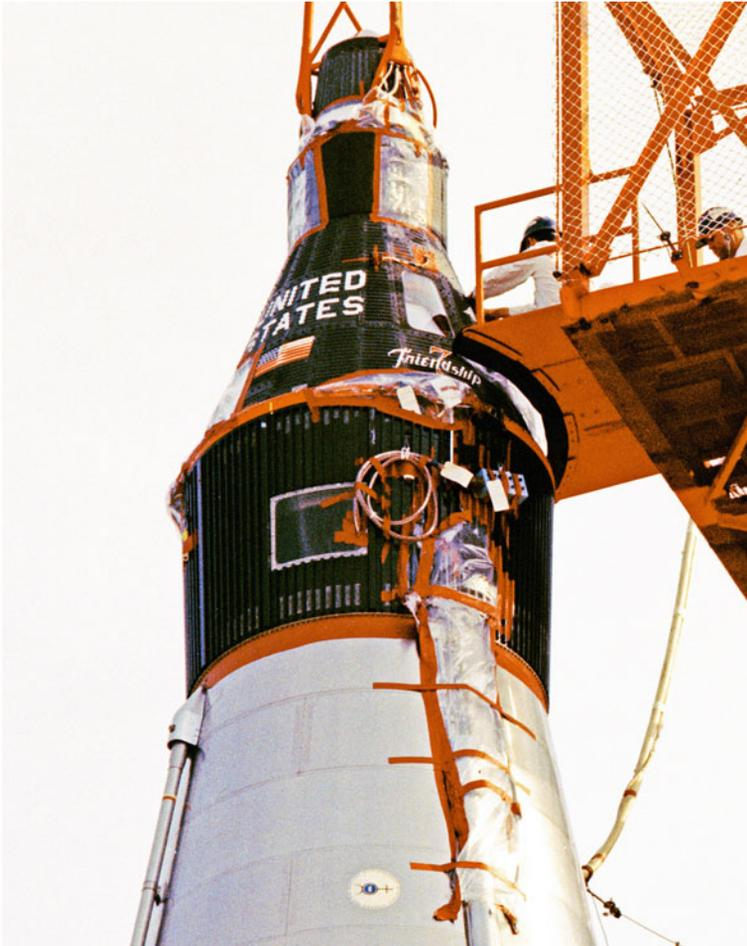
22 January 1962: Mercury capsule No. 13 mounted atop Atlas 109D on Launch Pad 14 with the egress facility extended to the capsule. (Photo: NASA/KSC)
